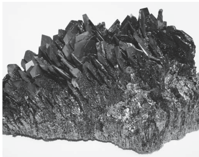
FIGURE 19.7 SiC produced by the Acheson process.
