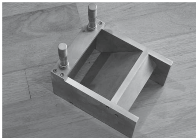
FIGURE 27.3 Typical doctor blade assembly.
