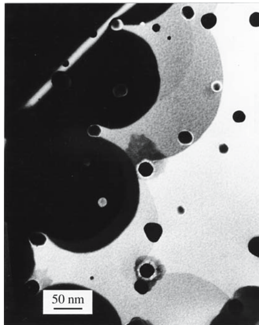
FIGURE 13.20 Plan view TEM images of steps on \text{MgAl}_2\text{O}_4 and \text{Al}_2\text{O}_3 ; the steps occur when the thickness of the TEM sample changes abruptly.
