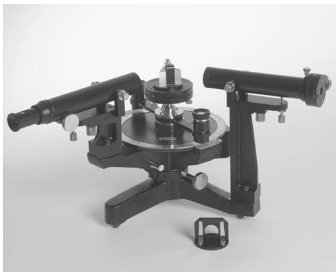
FIGURE 36.7 Goniometer-style refractometer.
