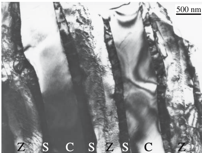
FIGURE 15.18 A CoO/ZrO 2 eutectic after solidification and subsequent oxidation. Z, ZrO 2 ; C, CoO; S, Co 3 O 4 (spinel).
