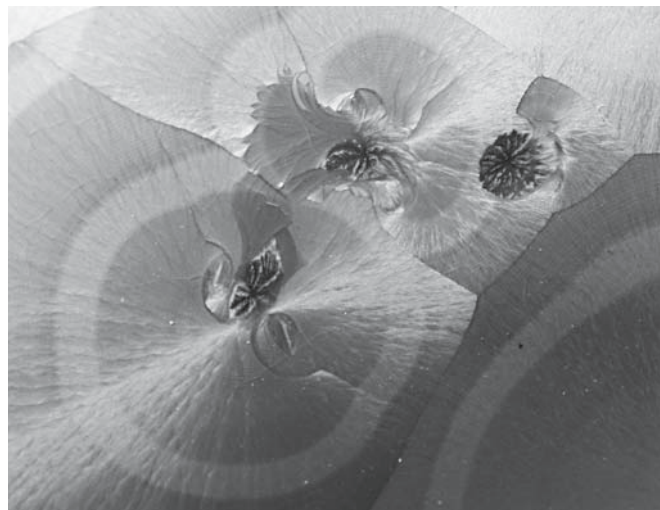
FIGURE 21.15 Illustration of spherulitic crystallization in a glass.
